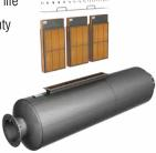
The ZX-Series' slide-in feature, which does not rely on moving parts or a complex loading apparatus, allows users to safely and easily lift/install/remove catalysts. In addition, the housing's customizable configuration makes it possible for catalysts to be inserted vertically or horizontally.
