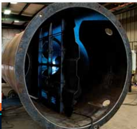
Integrated catalyst and silencer technology
