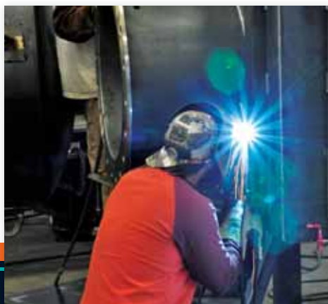
ASME Section 9 quality welds and reinforcement
