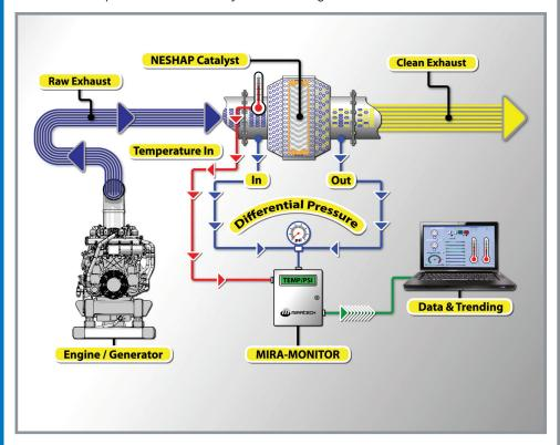
The MIRATECH MIRA-MONITOR includes the technology equipment needed to monitor and record inlet temperature and differential pressure to comply with NESHAP CPMS requirements. Users can configure and extract logged data reports using the computer software provided and also provided credible evidence of continuous compliance with NESHAP regulations.
