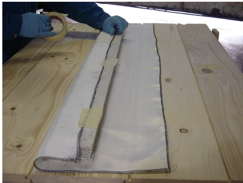
Figure 29: Assembling Expansion Mat Bundle
