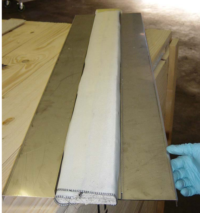
Figure 30: Expansion Mat Bundle Installed on Tray
