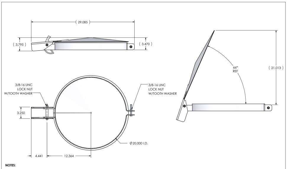
• STACK SHOULD EXTEND ABOVE CLAMP APPROXIMATELY 0.25" WHEN PROPERLY INSTALLED
