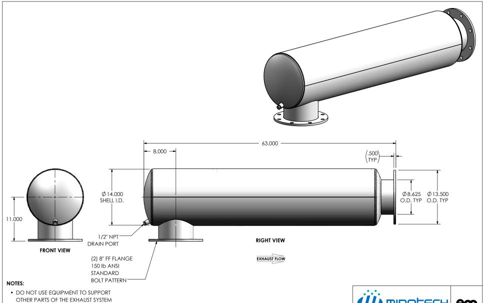
WITHOUT PROPER REINFORCEMENT
