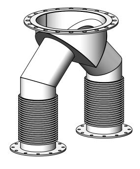
• DO NOT USE EQUIPMENT TO SUPPORT OTHER PARTS OF THE EXHAUST SYSTEM WITHOUT PROPER REINFORCEMENT
